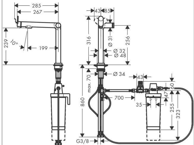
**Aqittura M91****FilterSystem 240, 1jet, Starter Set**Oberfläche: **Edelstahl Finish** Artikelnummer: **76802800**
